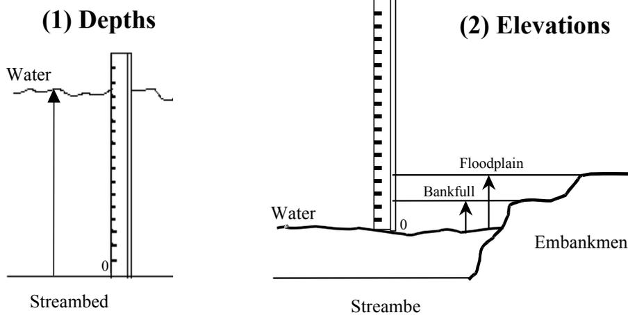
**Figure 2.** Depth and elevation measurements used in the detailed channel methods.
