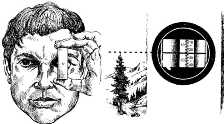
**Figure 3.** Slope measurements with a handheld clinometer.
