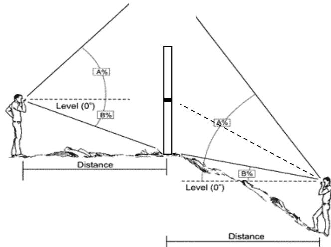
**Figure 4.** Adjusting for ground to eye height when taking clinometer measurements.
