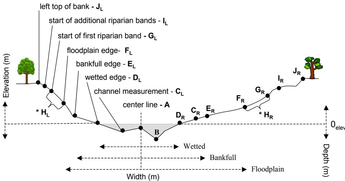
**Figure 1.** Cross-sectional measurement points for SHIM stream surveys.
