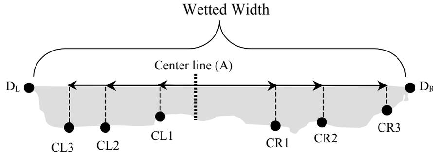
**Figure 5.** Incremental channel width measurements taken from the channel center line.
